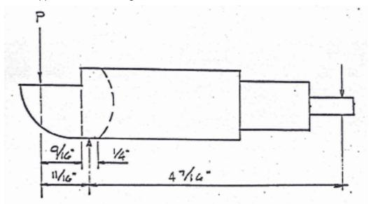
The load P is the load to be resisted - the limiting strength is thru the hole in the tongue. The reactions are:
